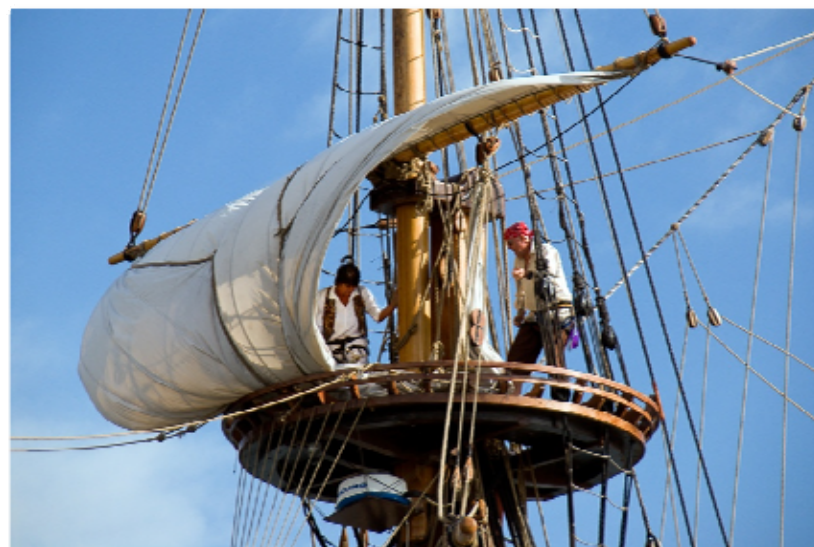
Figure 21 – Crew volunteers Maggie Brenner and Van Wells are working in the fore top...above the lower mast and below the topmast...preparing the fore topsail for use. Also visible is the fore top yard which is the horizontal spar the sail is attached to. Photographer – Alistair Gillanders.
