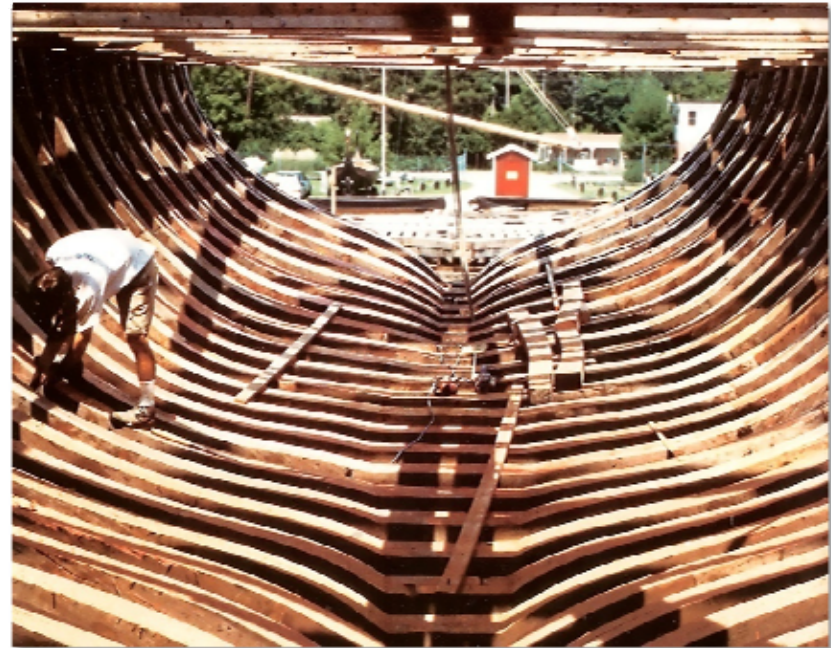
Figure 23 - In this view, aft looking forward, Patrick Flynn is smoothing the frames into fair curves, a process known as "fairing" the frames. Photographer – Jim Durborow
